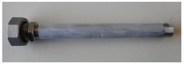
Adjust the large stainless steel nut to give a 2mm section of unthreaded stainless steel tube to be visible above the heatsink. This will provide for some compression of the large upper o-ring, & better sealing.
