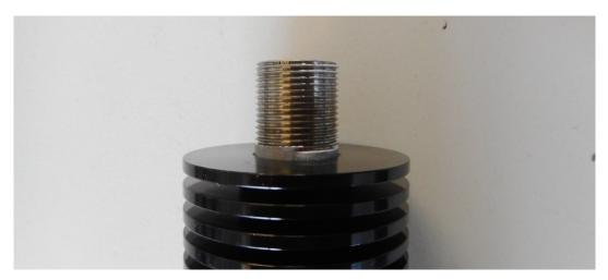
This picture shows the 2mm gap that has been adjusted using the large stainless steel nut. The 2mm gap should be set to the minimum thread gap. You can see a step down to where the thread stops. Set the 2mm gap here.
